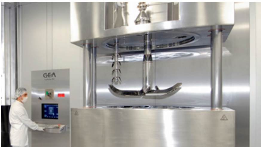
Gambar 5.16 Collette–Gral granulator: mixing shafts dan bow (sumber: http://www.gea.com/en/products/gral-ultimagral.jsp )
