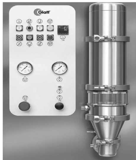
Gambar 5.22 Tabletop fluid bed processor (Courtesy of the Glatt Group sumber: Handbook of Pharmaceutical Granulation)
