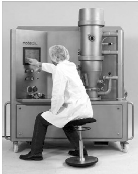
Gambar 5.21 Fluidized-bed granulator skala lab. (Courtesy of Heinen, Germany, disunting dari Handbook of Pharmaceutical Granulation)
